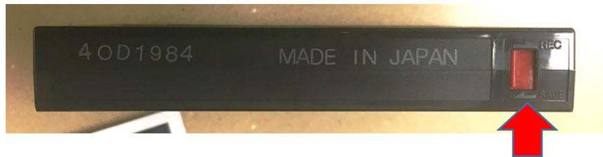
It is recommend that you protect your home video tape from being overwritten or erased by sliding the write protection tab to the **SAVE position**, located on the back edge of the tape. The photo above shows a tape that is protected.
