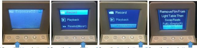
4 Press the Menu button 5 Press the Down button 6 Press the Enter button 7 Press the Enter button and highlight Rewind
