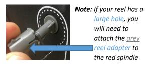
3 Route the film along the dotted line that is printed on the chassis
